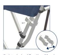
B. Attach the Alloy Knuckle, clamping the Bimini and Rocket Launcher Frames together (as shown). Repeat on opposite side. Adjust to preferred height.
