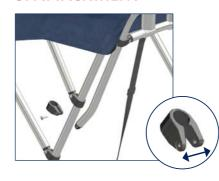
A. Open the Knuckle enough to wrap around the bimini upright. Connect to the assembled Rocket Launcher and screw in place. Repeat on opposite side.
