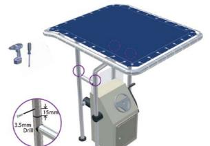
C. Attach the CANOPY SECTION to the **BASE SECTION**. Secure permanently using self tapping screws (supplied) (As shown in the diagram)
