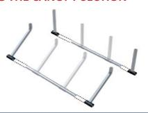
**B.** Insert side frames into the support poles. The support pole housing the 'T' joiners should be closest to the side frame bend.
