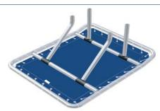
E. Lay out the canopy fabric topside down and place the inverted frame over it. Lace nylon cord through the eyelets and frames, Ensure its evenly threaded and tight.
