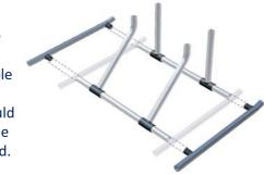
C. Insert the **U frames** onto the ends of both side frames.
